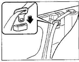
To secure the passenger's seat belt when not in use, insert the seat belt tongue into the slot.
