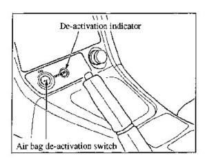
The air bag de-activation switch turns off the passenger-side air bag. Make sure the passenger side air bag deactivation switch is in the ON position except when a passenger fitting the previous categories occupies the front passenger seat.
