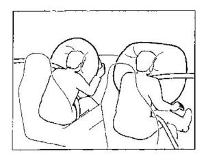
The air bags will function only once. After that, the air bags will not work again and must be replaced.
